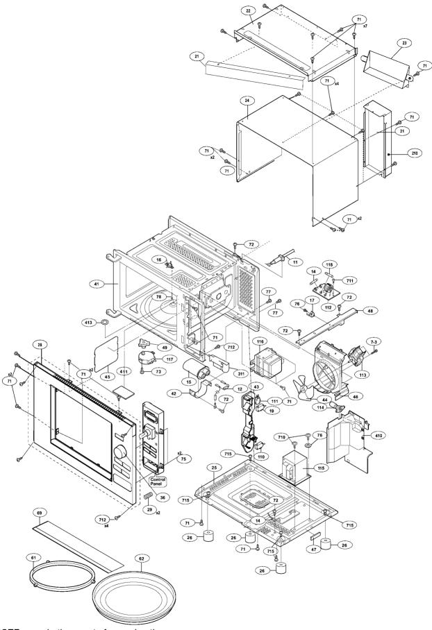
NOTE: In the event of removing the turntable motor cover this part should be refitted using screw connection: LX-EZA045WRE0 (710)
